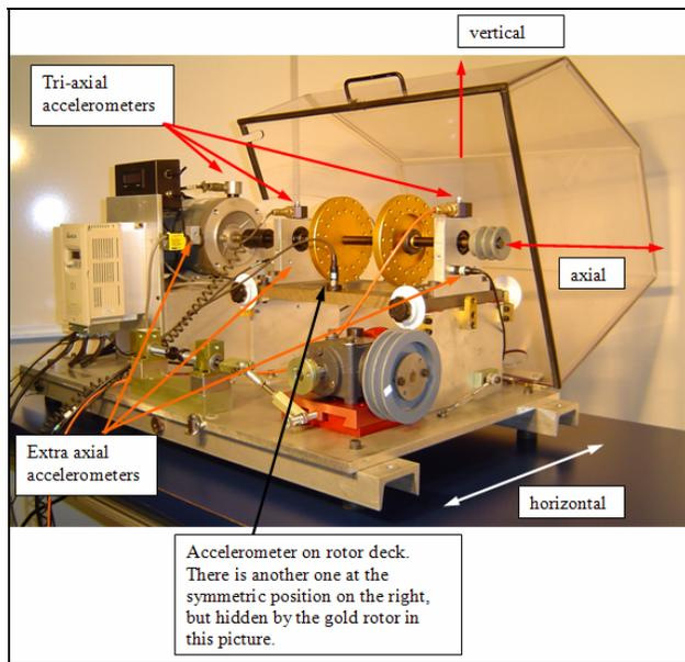
Figure 2. Accelerometers on Motor & Bearings.
