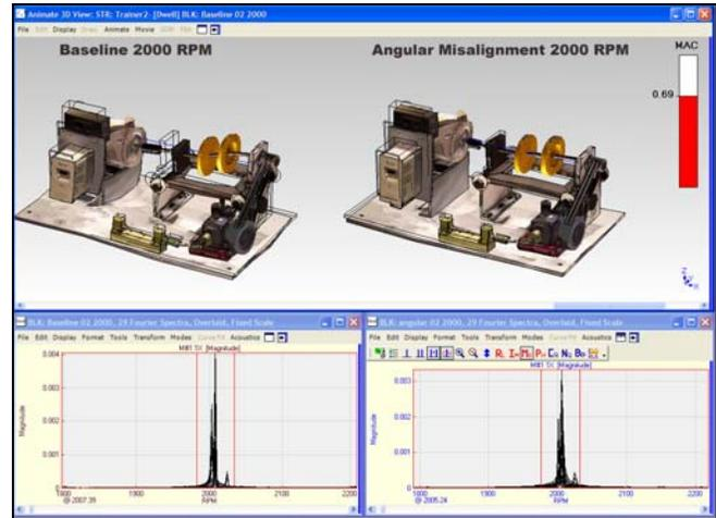
Figure 6. Angular Misalignment - 2000 RPM.
