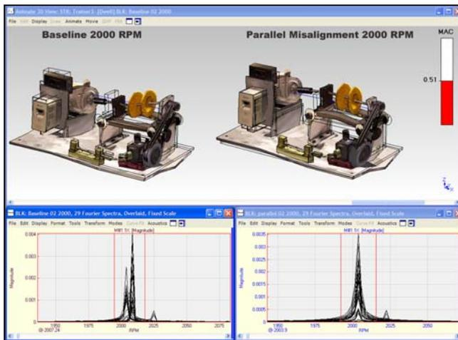
Figure 5. Parallel Misalignment- 2000 RPM.
