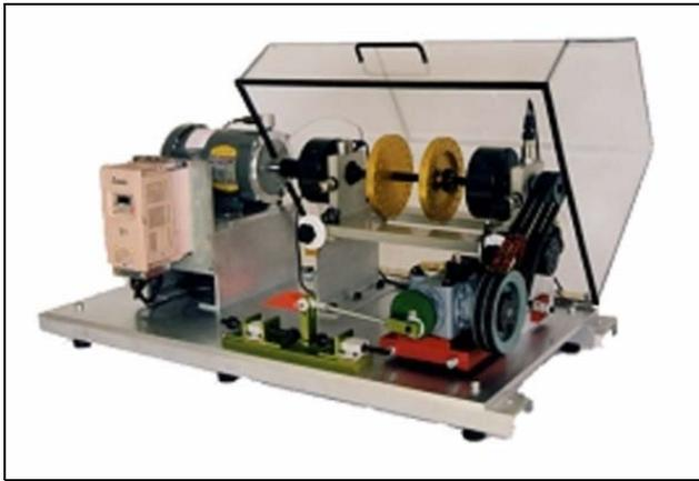
Figure 1. Machine Fault Simulator.
