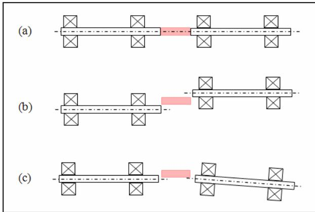
Figure 4. Parallel (b) & Angular (c) Misalignment.
