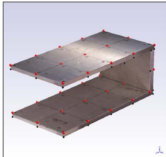
Figure 1. Beam Structure Showing 33 Test Points.
