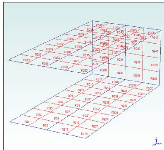
Figure 2. FEA Model with 80 Quad Plate Elements.
