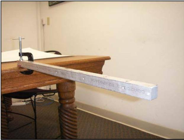
Figure 3. Aluminum Bar Clamped to a Table Top.
