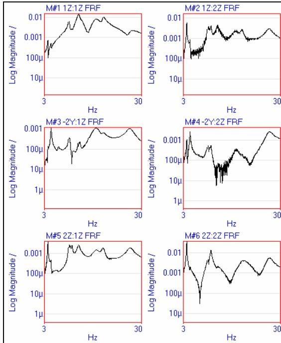
Figure 1. 3 by 2 FRF Matrix from Z24 Bridge.
