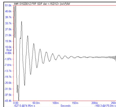
**FIGURE 1. Impulse Response with Leakage.**
