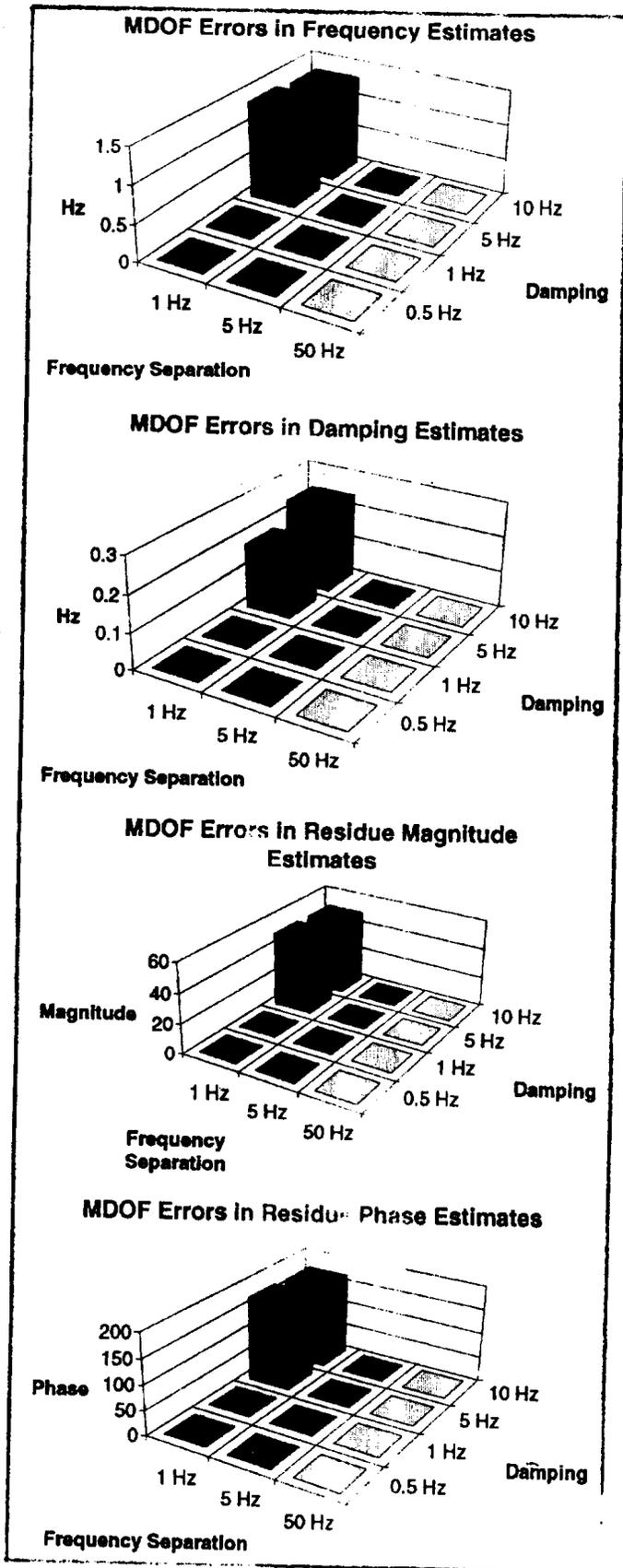
Figure 6. MDOF Curve Fitting Errors: Cases 1-12
